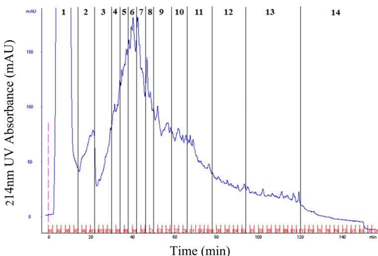
**Figure 2. SCX fractionation of peptides mixture from rice mature pollen grain.** According to the 214 nm UV absorption peak, the peptides mixture can be pooled into 14 fractions for LC-MS/MS analysis.
